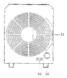
21 - Voltage change cover22 - Supply cable input23 - Grounding screw
