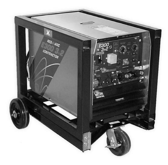
2000 Watts AC Auxiliary Power Rugged Tubular Pak-Lok-Frame™ Extreme-Duty™ Stainless Steel Construction 350 Amps Output at 34 Volts and 20% Duty Cycle Available as 4Pak™ and 6Pak™ Multioperator Systems
