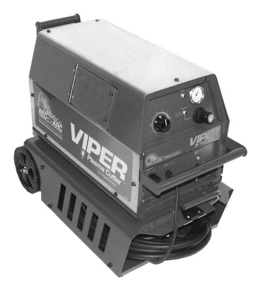
Cutting Capacity up to 3/4" 28 IPM Cutting Speed at 1/2" High Speed Inverter Technology 60 Amps of Output at 50% Duty Cycle PCT 80 Plasma Torch without High Frequency
