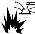
**WELDING SPARKS can cause fire or explosion.**
