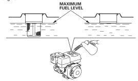
3. Refuel carefully to avoid spilling fuel. Do not fill the fuel tank completely. It may be necessary to lower the fuel level depending on operating conditions. After refueling, tighten the fuel filler cap securely.
