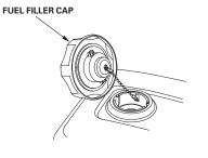
Add fuel to the bottom of the maximum fuel level limit of the fuel tank. Do not overfill. Wipe up spilled fuel before starting the engine.
