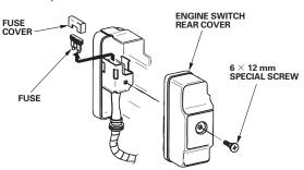
Frequent fuse failure usually indicates a short circuit or an overload in the electrical system. If the fuse burns out frequently, take the engine to a Honda servicing dealer for repair.
