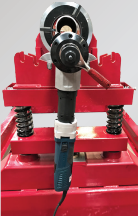
Standard Cutting & Bevelling tools for KPI1-KPI2-KPI3-KPI4-KPI5 Machines
