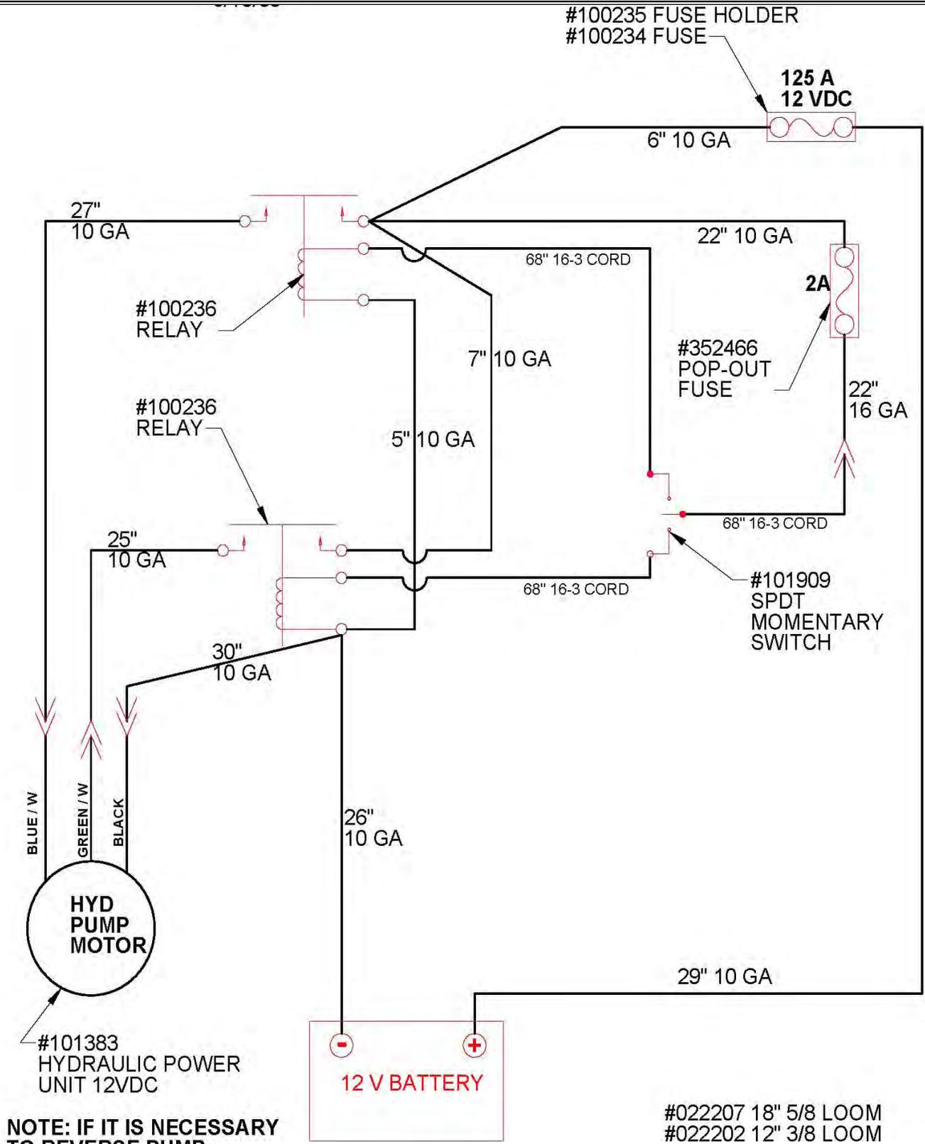
**NOTE: IF IT IS NECESSARY TO REVERSE PUMP DIRECTION, SWITCH BLUE/W & GREEN/W WIRES FROM PUMP MTR.**
