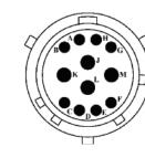
12-Pin ArcLink Wire Feeder & Digital Accessory Connectivity
